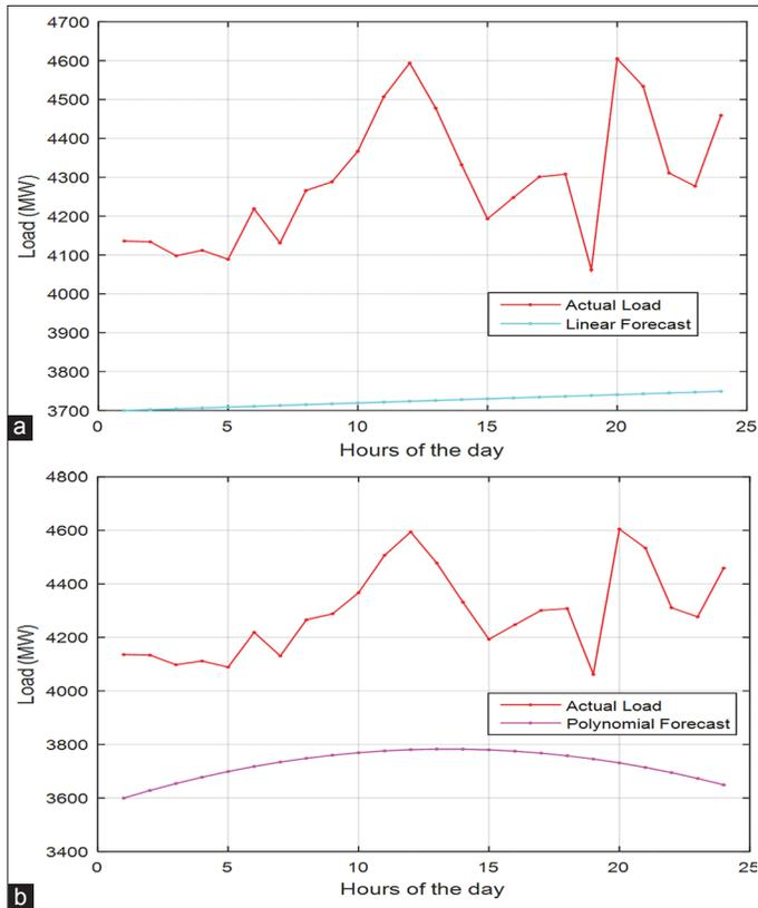
**Figure 5:** Comparison of actual and forecasted load curve of Artificial Neural Network model for 31<sup>st</sup> March-2017
