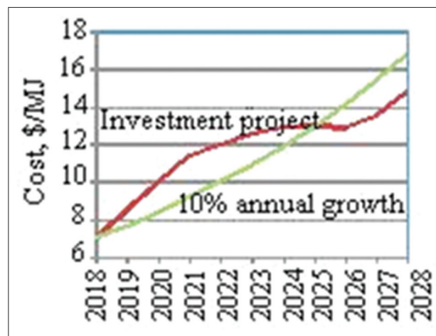
Figure 3: Comparison of the heat energy tariff under the investment project and without the upgrade, given 10% annual forecast growth
